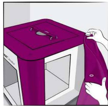
Install and secure the top with 4 large white hand screws.
