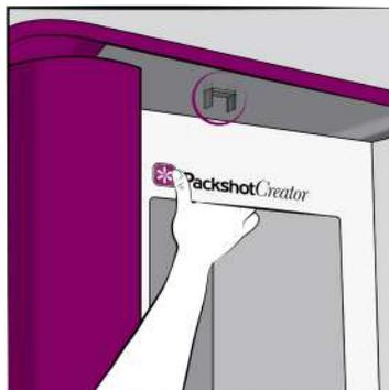
Replace the top. Make sure to orient the top so that the camera strap goes left to right when viewed from the front. **Note:** Align the acrylic panels with the holding brackets at the top to hold them in place.
