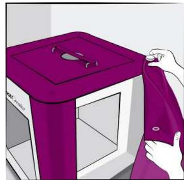
Fix the top using 4 white hand screws. If you use the acrylic side diffusion panel with the opening, remove the side wall and attach the reflective door cover for convenient side loading.
